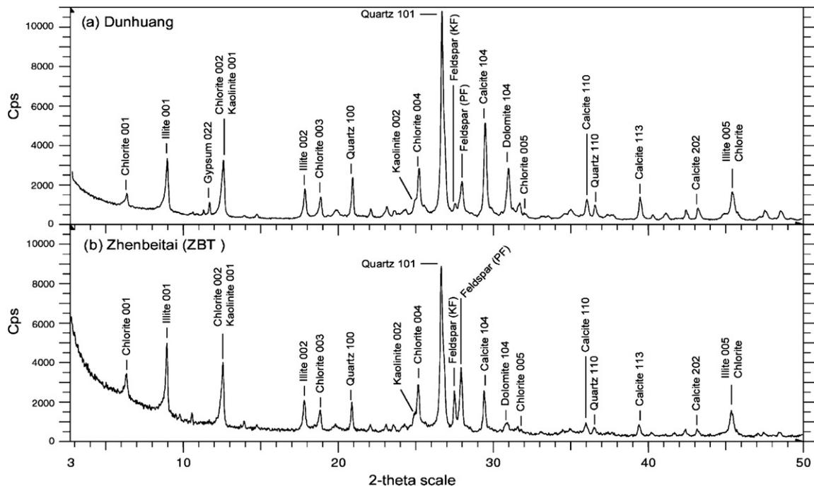
Fig. 2. Typical X-ray diffraction spectra of bulk aerosol samples collected at (a) Dunhuang and (b) Zhenbeitai.
