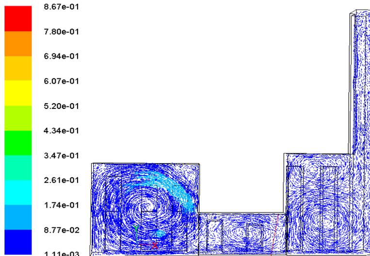
Fig. 4. Air movement in the plane of  $z = 3$  m.
