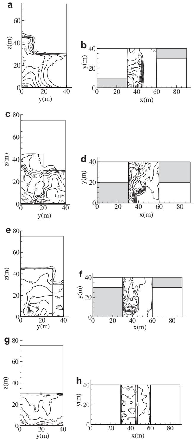
**Fig. 10.** Contours of the simulated normalized pollutant concentrations in different cases of non-uniform street canyons in planes 2 m from the leeward walls ((a), (c), (e), (g)) and at the pedestrian level 1.5 m above the road surface ((b), (d), (f), (h)). Figs. (a) and (b) are the simulated results of Case 2, (c) and (d) are the simulated results of Case 3, (e) and (f) are the simulated results of Case 4, (g) and (h) are the simulated results for the uniform street canyon Case 1.
