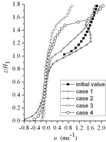
**Fig. 9.** The mean wind profiles in the four cases and the initial wind velocity values inside and above the street canyons. ■ – the initial value, + – the simulated results in Case 1, \* – the simulated results in Case 2, Δ – the simulated results in Case 3, and ○ – the simulated results in Case 4.
