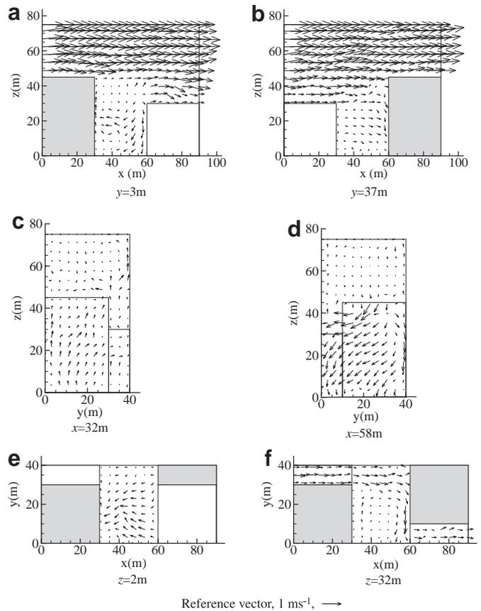
Fig. 8. The velocity vectors in (a) the longitudinal vertical plane in the stepdown section,  $y = 3$  m, (b) the longitudinal vertical plane in the stepup section,  $y = 37$  m, (c) the lateral vertical plane at 2 m from the leeward wall,  $x = 32$  m, (d) the lateral vertical plane at 2 m from the windward wall,  $x = 58$  m, (e) the horizontal plane near road surface,  $z = 2$  m, (f) the horizontal plane 2 m over lower building top,  $z = 32$  m for Case 4.
