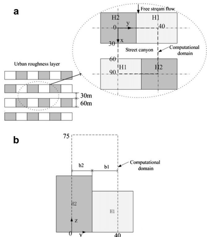
**Fig. 1.** Layout of non-uniform street canyon, in top view (a) and side view (b). The area depicted with dashed lines is the computational domain. Deep gray areas indicate the high buildings.  $H_1$  and  $H_2$  are the heights of the high building and low building, respectively.  $b_1$  and  $b_2$  are the lengths of the low and high buildings occupied in the computational domain, respectively.
