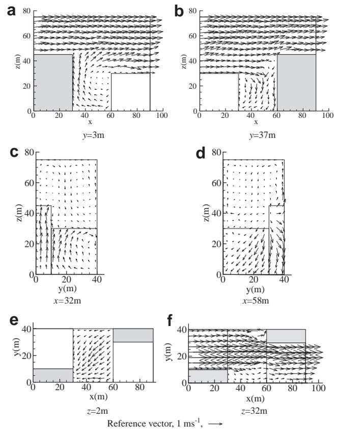
Fig. 5. The velocity vectors in (a) the longitudinal vertical plane in the stepdown section,  $y = 3$  m, (b) the longitudinal vertical plane in the stepup section,  $y = 37$  m, (c) the lateral vertical plane at 2 m from the leeward wall,  $x = 32$  m, (d) the lateral vertical plane at 2 m from the windward wall,  $x = 58$  m, (e) the horizontal plane near road surface,  $z = 2$  m, (f) the horizontal plane 2 m over lower building top,  $z = 32$  m for Case 2.
