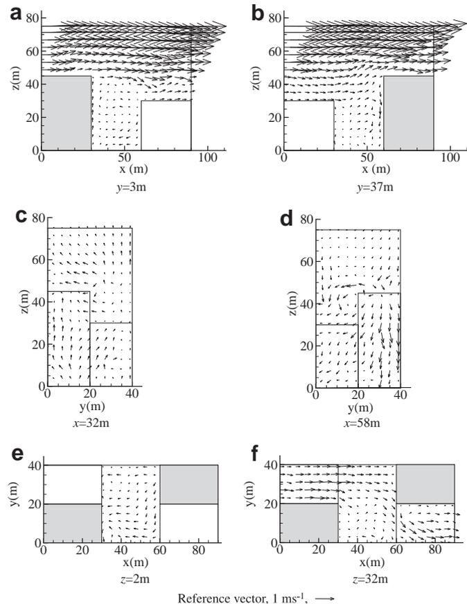
Fig. 7. The velocity vectors in (a) the longitudinal vertical plane in the stepdown section,  $y = 3$  m, (b) the longitudinal vertical plane in the stepup section,  $y = 37$  m, (c) the lateral vertical plane at 2 m from the leeward wall,  $x = 32$  m, (d) the lateral vertical plane at 2 m from the windward wall,  $x = 58$  m, (e) the horizontal plane near road surface,  $z = 2$  m, (f) the horizontal plane 2 m over lower building top,  $z = 32$  m for Case 3.
