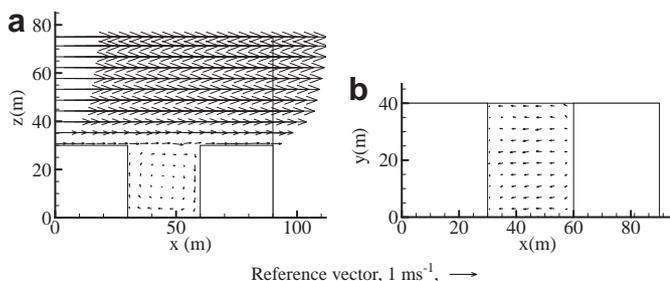
Fig. 4. (a) The velocity vectors in the longitudinal vertical plane at  $y = 20$  m for Case 1, (b) the velocity vectors in the horizontal plane at  $z = 2$  m for Case 1.
