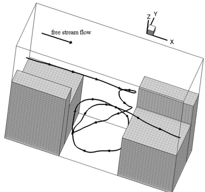
Fig. 6. A typical stream line in the non-uniform street canyon of Case 2.
