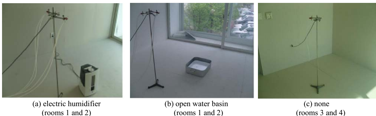
Fig. 4. Humidifying conditions in the mock-up rooms.
