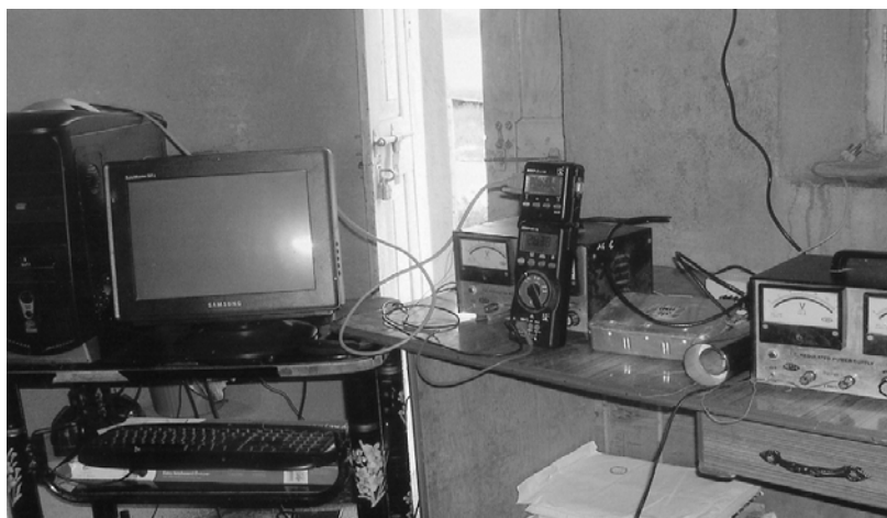
Fig. 2. Cluster air ion counter: with power supply, fan, electrostatic shield, digital voltmeter, data logger, and personal computer.
