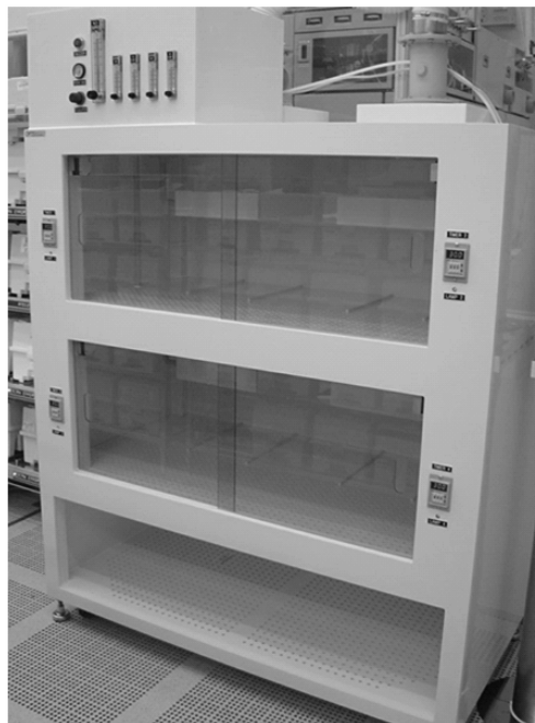
Fig. 6. Photo of a wafer storage cabinet for capturing the outgassing acid gases.(Dimensions: 1.4 m by 1.5 m by 0.75 m, circulation air flow rate = 4200 L/min).
